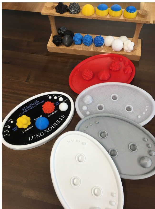
Top: UV Printing text and graphics to the face plate. Bottom: 3D printing allows quick variance in color and materials.
